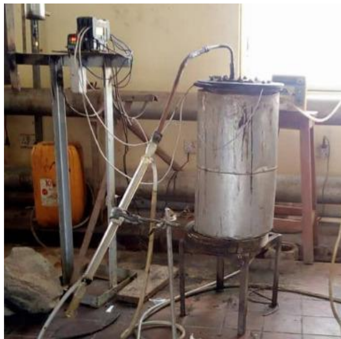
Fig. 3. Fixed Bed Reactor used for pyrolyzing feedstock.
